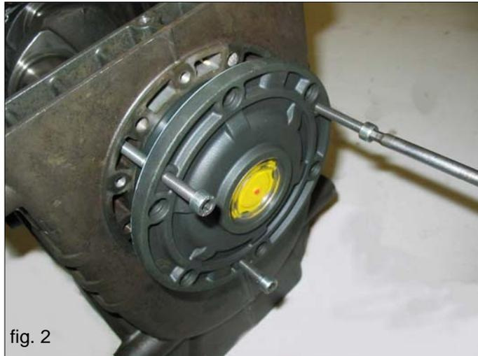
Push the piston guides and connecting rods forward in order to facilitate the lateral extraction of the pump shaft.
