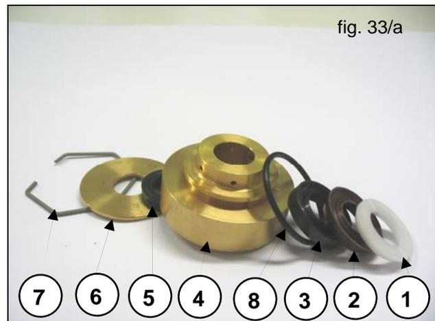
**2.2.4 Piston unit disassembly**
